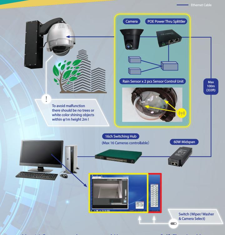
Max 16 Cameras can be connected. You can program Self-Cleaning Menu. (E.G. at 8:00a.m. and 14:p.m. washer runs 2 times and wiper runs 5 times.)
