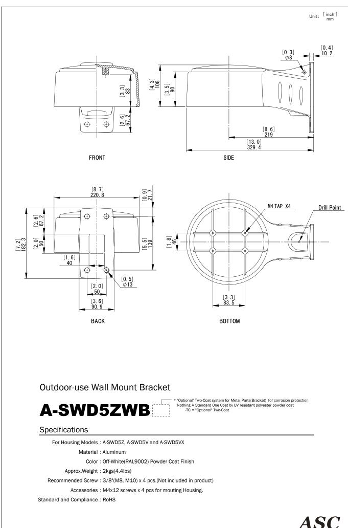
\* "Optional" Two-Coat system comprises 1coat = powder coating primer(Epoxy base) and Top coat = UV resistant(Polyester base) powder coating based on our standard.
