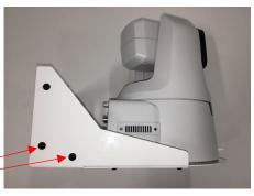
Fix 3 Screws temporarily, check center of 2 Holes, fix all 5 screws completely. **Example 2)** Canon CR-N500 Bracket(INVERTED)
