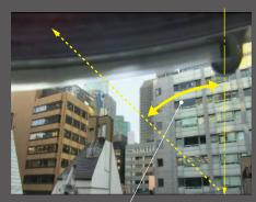
Vertical Viewing Angle 35° Tilt Up +20° Center of Lens Tilt 0° Center of Lens Pan Left 20° Viewing Upper Housing (Tilt UP+20°) Note : In case of Tilt Down - 8°, No Upper Housing Visible within Tilt 300° Area.
